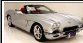
1962 Corvette Retro (C5). CRC carbon fiber panels on 2000 body, chassis, and suspension. Sebring Silver with Red interior! Dynamic show car.
